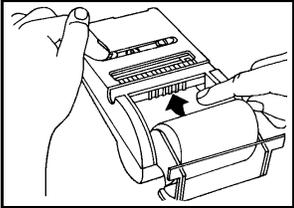
Hold down the
