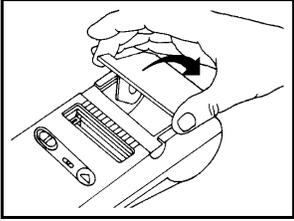
Open the paper roll door and remove the used paper roll core.
