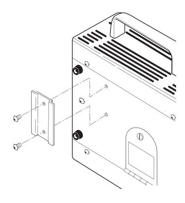
Figure 3-2 Dovetail rail mount bracket attachment (male bracket mounting on light source)
