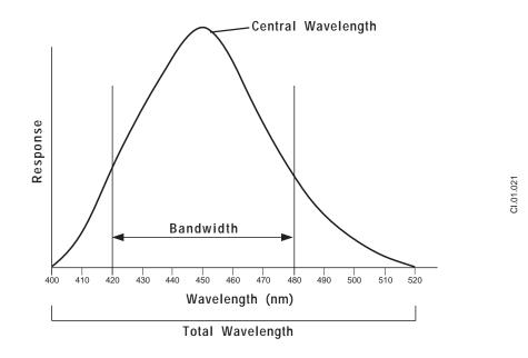
Figure 4-3 Typical Phototherapy Light Meter Response
