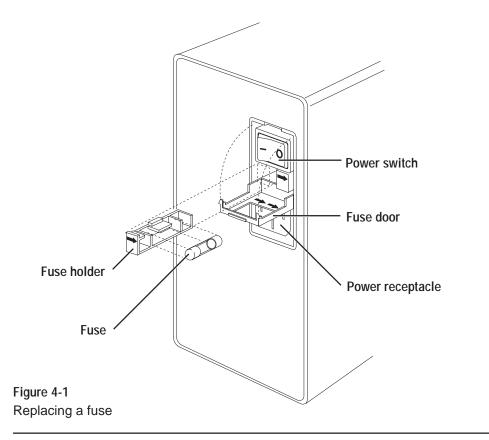
4. Replace fuse with the correct replacement fuse.
