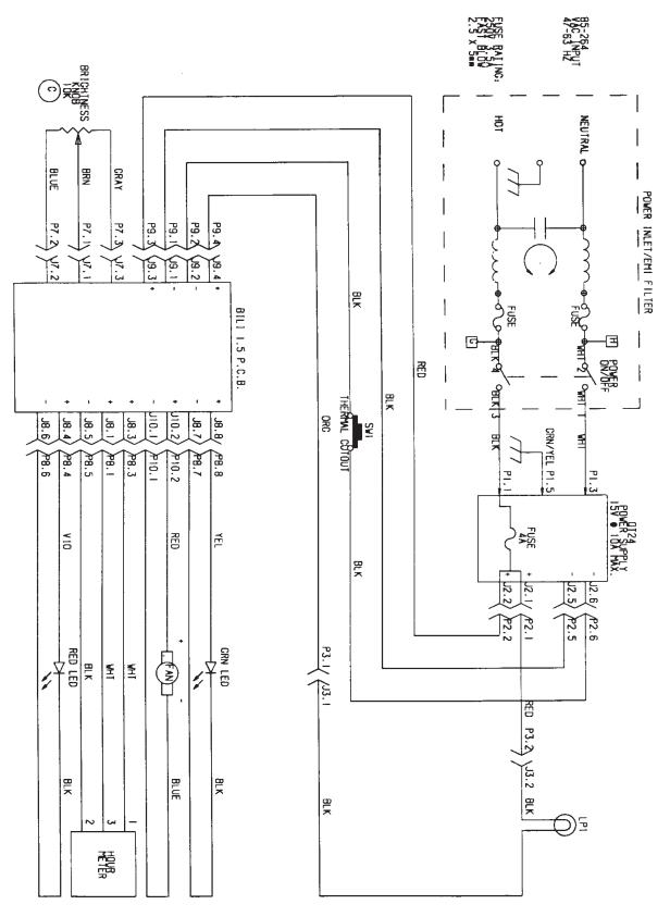
Figure 4-7 Wiring Diagram
